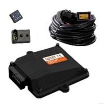
Designed for all types of 5-6 Cylinder vehicles. Very lightweight, shock resistance, waterproofs plastic housing, intelligent with OBD option, auto calibration and auto map correction, Gas injector heating and diagnostic, valve protection, real time diagnostic of components, best calibration result with OBD connection.
